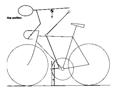
seated position. At extremely high pedaling forces, the rider comes out of the saddle to straighten the load path for his arms which allows them to effectively resist the loads created by the much stronger leg muscles. The diagram of the lever system in Figure 1 is no longer accurate at this point; the rest of the rider becomes a complicated system of levers as well.
